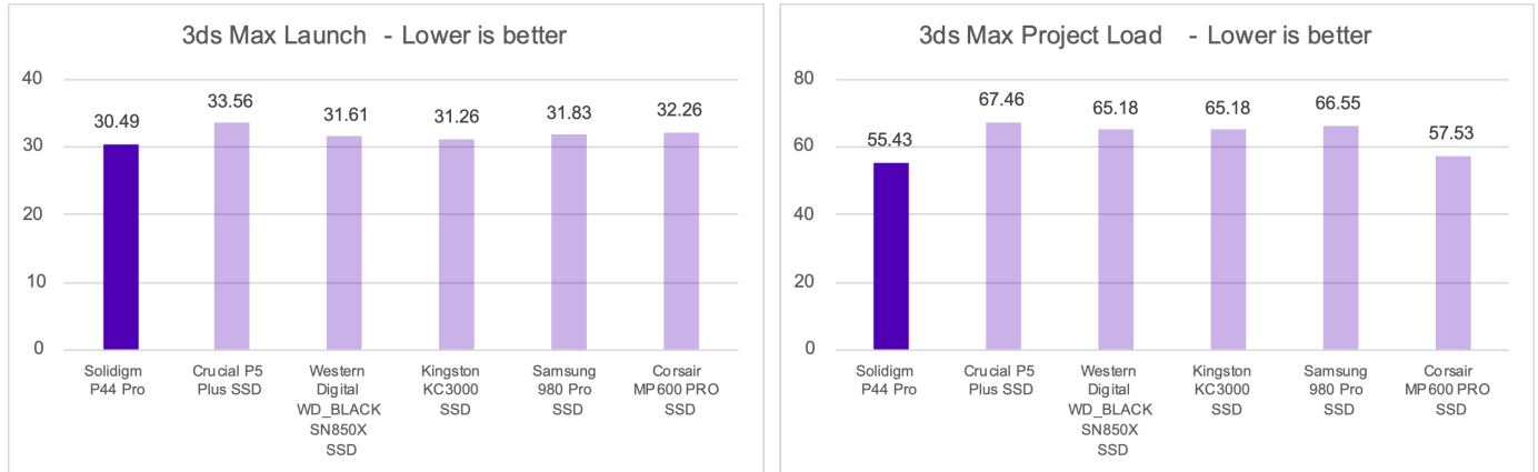
[Figures 14A and 14B. Application launch and project load in Autodesk 3ds MAX - Laptop]
